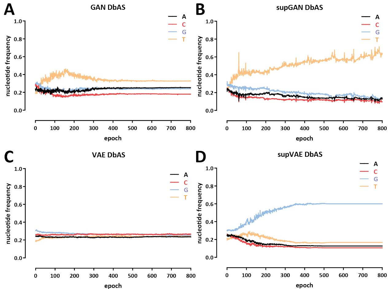
**Figure 13. Base pair composition throughout training for the DbAS tuning method.** (A) Generative Adversarial Networks (GAN) + DbAS; (B) Supervised Generative Adversarial Networks (supGAN) + DbAS; (C) Variation AutoEncoders (VAE) + DbAS; (D) Supervised Variation AutoEncoders (supVAE) + DbAS.
