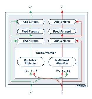
*Figure 2.* Cross transformer encoder. Norm indicates the layer normalization. Feed Forward indicates the position-wise linear layer.
